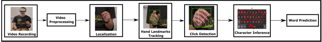
Figure 3: Figure shows the steps involved in the execution of the Hidden Reality attack model. An adversary captures the video footage of a targeted user while the user is performing typing operation on their virtual screen. Region of interest is obtained by localizing the typing hand and tracking the hand landmark points on the preprocessed video. By mapping the tracked hand pixel location coordinates obtained in the click detection step onto the known keyboard geometry, the typed text gets inferred.
